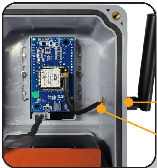
**STEP 1** Thread antenna onto bulkhead. Hand-tighten until snug
