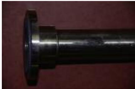
**Figure 1. Galling on the stem due to an oversized valve or operating the PRV too close to set pressure.**
